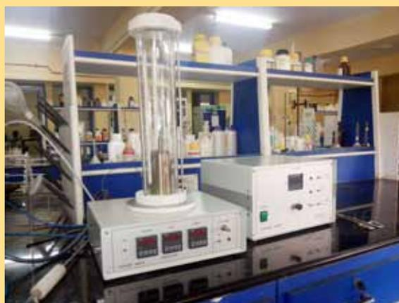
Fig.2: Limiting oxygen Index test
