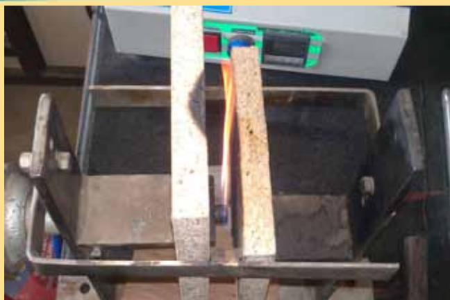
Fig.1: Flammability test of particle board
